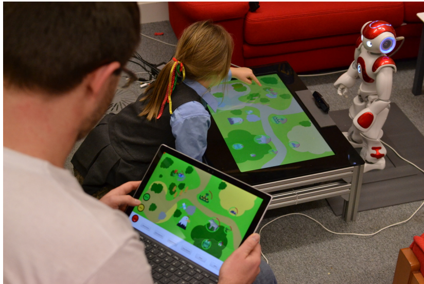
Figure 2: The setup used in the study: a child interacts with the robot tutor, with a large touchscreen sitting between them, displaying the learning activity; a human teacher provides guidance to the robot through a tablet and monitors the robots learning.
