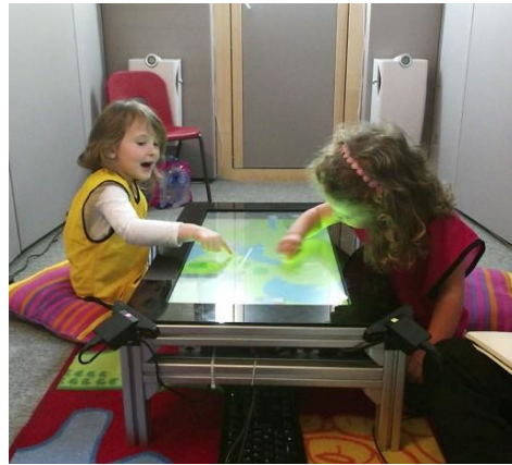
Figure 1: Setup used to evaluate the effectiveness of face detection in a spontaneous interaction between two children. Children are facing each other and sit on cushions. Each child wears a bright sports bib, either purple or yellow, to facilitate later identification. Cameras are mounted at position where the robot would be observing the children.
