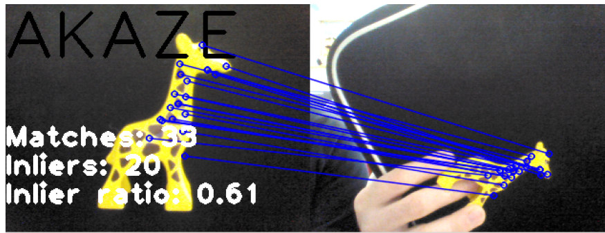
Figure 3. Image showing target on the left, with an object being tracked through a rotation on the right using A-KAZE.
