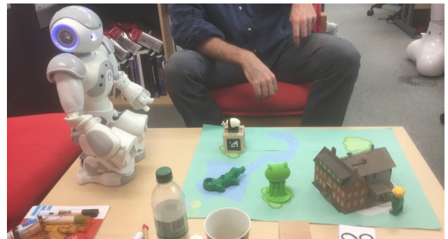
Figure 1. A close proximity interaction setup, typically found in human-robot interaction and cognitive robotics scenarios. While the number and nature of objects varies from one experiment to another, key scene characteristics are usually constant: relatively small objects (e.g. largest side being less than 10 cm), presence of occlusions, limited working space, and the presence of both textured and texture-less objects.
