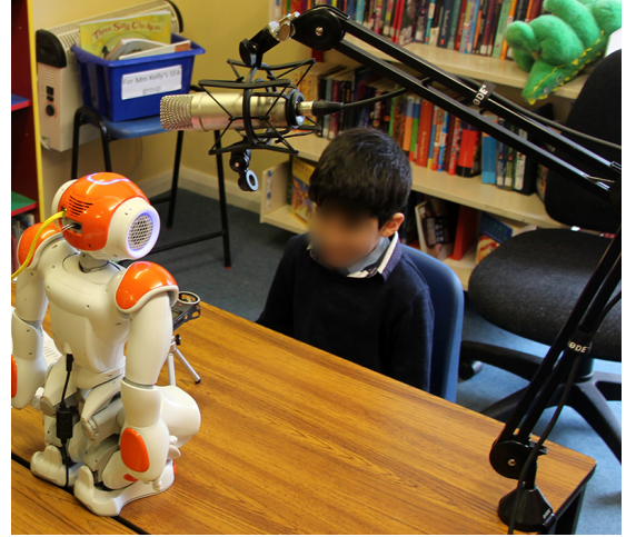
Figure 1: Equipment layout for recording children in a school. The Aldebaran NAO is turned on (but not moving) and records to a USB memory card. The studio microphone and portable microphone record simultaneously.
